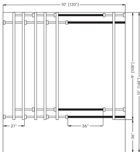
Overhead pullout racks require double the space of Spacesaver units.
