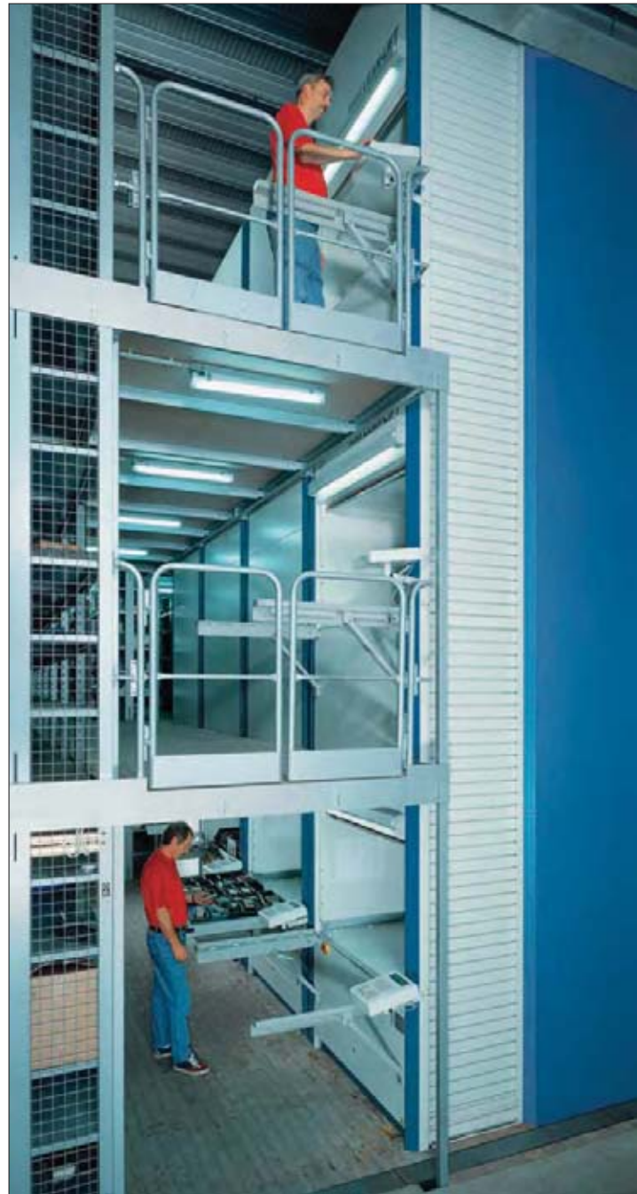
A Lean-Lift system with retrieval over several floors
