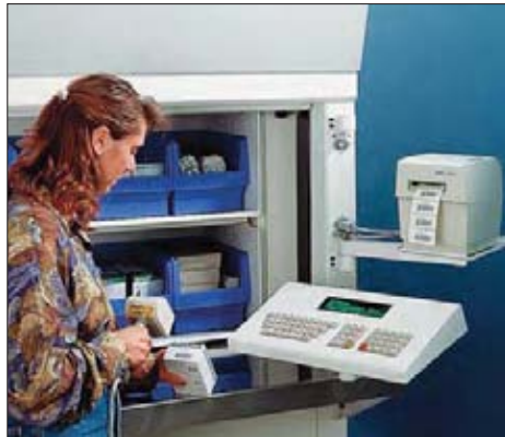
Recording the article number when goods are stored and display for control purposes
