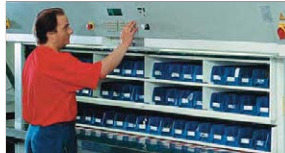
Small parts storage in plastic containers
