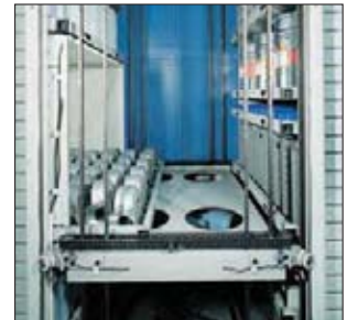
The extractor pulls the container...
