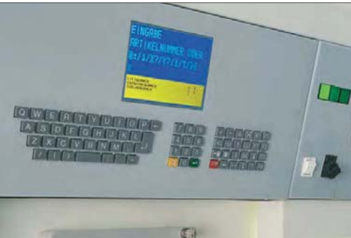
The new control keyboard of the Hanel Rotomat with CSTN panorama color display (optional)
