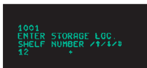
Hanel's automated load imbalance indicator UL 2 will recommend storage location
