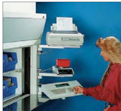
Central arrangement of all the peripheral units needed for order picking
