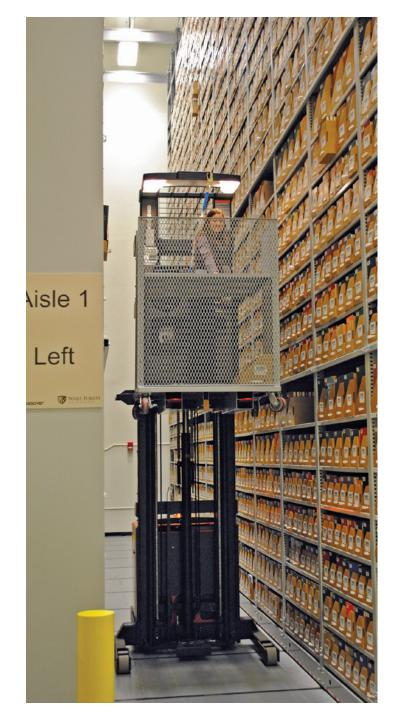
Integrated guide wire: when the bays open up and give someone access to the aisle, the forklift is centered on a guide wire, which keeps it on course. This means a user cannot run off course and into the shelving system.
